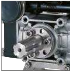
Cardano 1" \frac{3}{8} 1" \frac{3}{8} universal shaft
