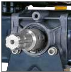
Cardano 1" \frac{3}{8} 1" \frac{3}{8} universal shaft
